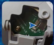
Connect customer supplied ethernet cable to "POE IN" and close the door.
