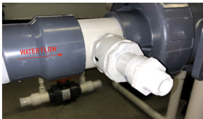
Inlet water pitot tube – notch facing upstream
