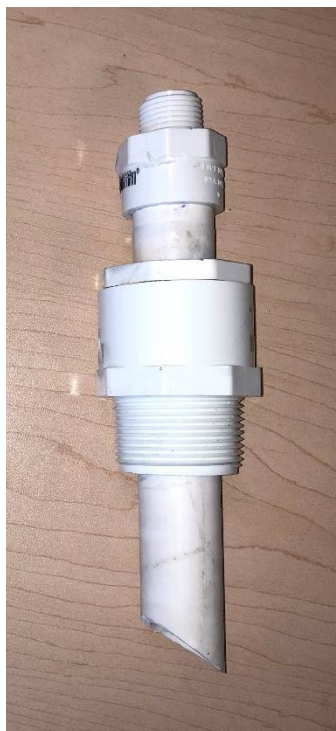
Pitot Tube – 2 5/8” For 3” pool piping
