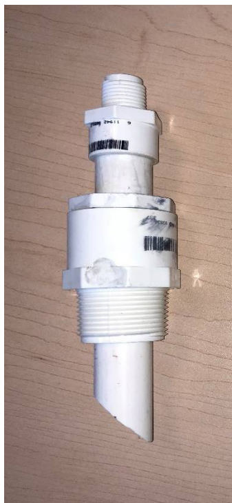
Pitot Tube – 1 7/8” For 2 ½” pool piping
